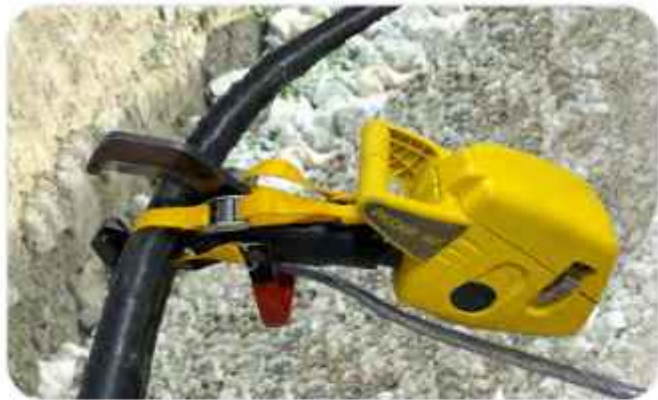
New cable retention strap for a successful remote-controlled cut for sure.
