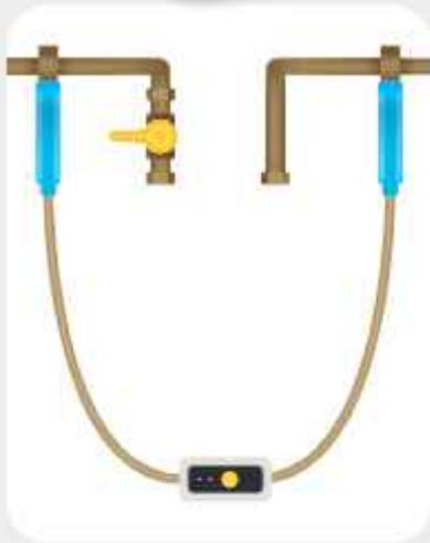
3 THE BYPASS MAINTAINS THE CONTINUITY WHEN THE OLD GAS METER IS REMOVING TO AVOID ANY SPARK
