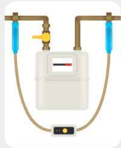
2 FIX THE 2 CLAMPS ON EACH SIDE OF THE GAS METER
