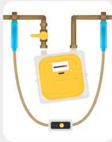
4 NEW GAS METER CAN BE INSTALLED
