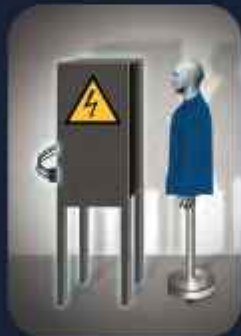
Determination of the clothing protection class according to the intensity of the electrical installation, in 2 classes : APC 1 (Arc Protection Class 1) (for 4 kA over 0.5 s at 30 cm) APC 2 (Arc Protection Class 2) (for 7 kA over 0.5 s at 30 cm) (European principle)
