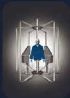
Determination of the ATPV and ELOM values of clothing expressed in cal/cm 2 (American principle)
