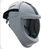
Arc-Flash APC 2 7kA / 0,5s ATPV 12 cal/cm 2 Beard : Integrated chin and lateral protection
